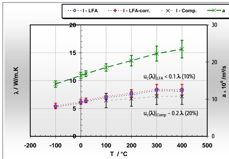
Figure 5. Thermal diffusivity and conductivity of a Mg-foam material. comparison between conductivity data from a comparative set-up and data calculated from flash based diffusivity data.
