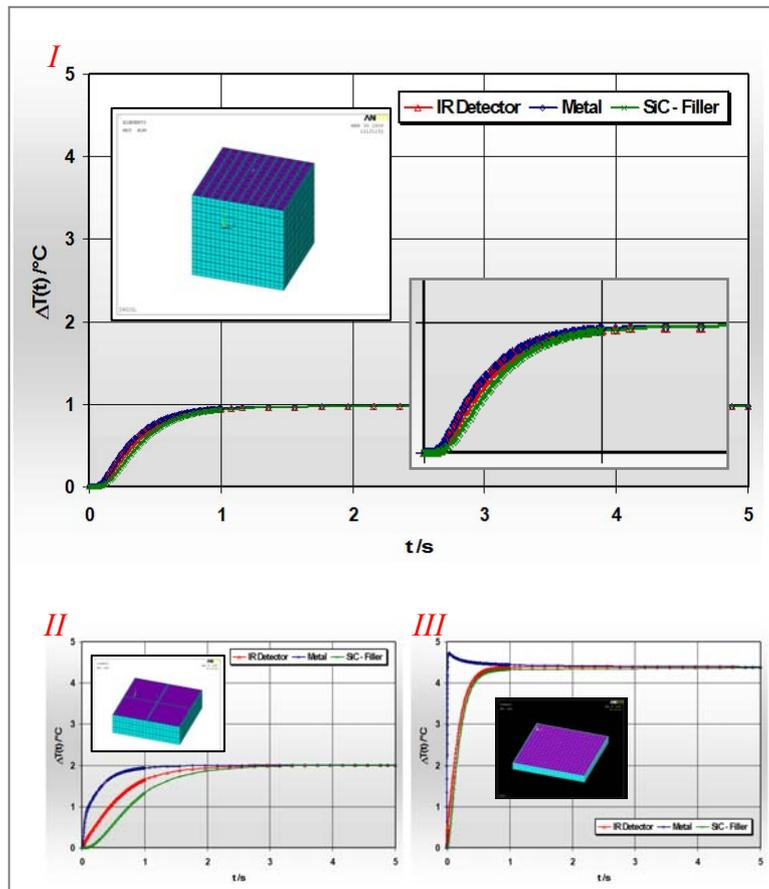
Figure 4. FE simulation of the transient temperature response of Mg-foam materials. Samples differ in their porosity. Porosity is filled with SiC.
