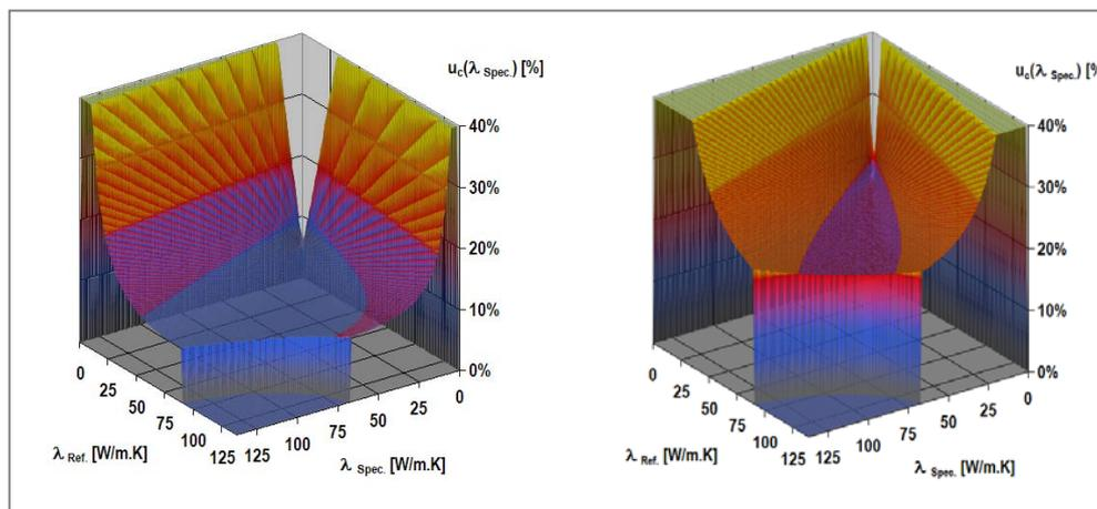
Figure 2. Comparative device: Equipment Specific Uncertainty  $ESU$  of thermal conductivity data.
