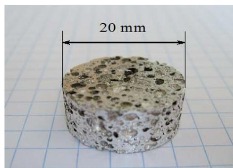
Figure 1: LFA sample of a Mg – foam material
